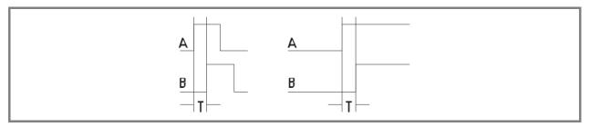
DIL switch S1 permits selection of 5 different times. The frequency is shown in brackets at which the phase displacement corresponds to 90°.
