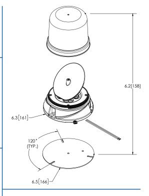
45° angled reflector driven by a quiet brushless magnetic drive system provides an exceptional warning beam without compromising reliability
